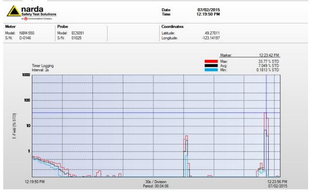
The values recorded that exceed 1% were measured inside the restricted areas of the roof in front of the antennas.
